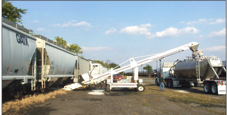
A train-to-truck sand transload facility at Williamsport, Pa. Each rail car has the same carrying capacity as 4-5 trucks.
